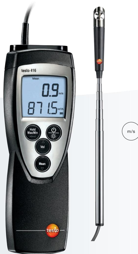
The testo 416 is a compact anemometer with a fixed vane probe. The measuring instrument is particularly suitable for flow velocity measurements in ducts thanks to the extendable telescope (max. length 890 mm, diameter 16 mm). The volume flow is directly shown in the display. For volume flow calculation purposes, the duct cross-section area can be conveniently entered into the testo 416. The timed and point mean value calculations provide information on the average volume flow.
