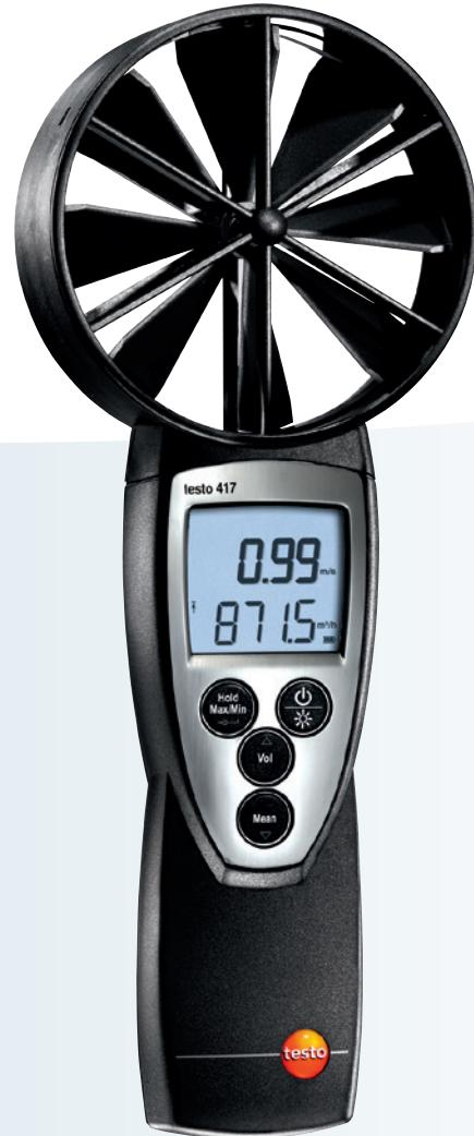
testo 417 is a compact, large-area anemometer with a built-in flow velocity / temperature vane. It measures flow velocity, volume flow and temperature. Thanks to the integrated measurement with the 100 mm vane, it is ideally suited for measurements at air input and output vents. The flow direction, i.e. blowing or sucking flow, is visible in the display. The optimum funnel set additionally allows measurements on ventilation grilles and disc outlets.
